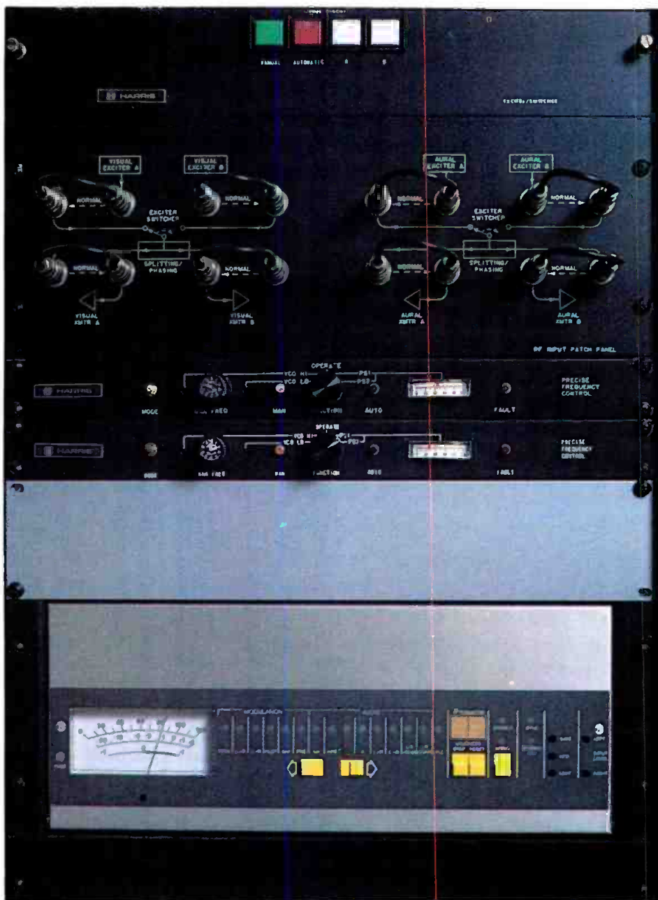
The stereo generator for WFSB-TV, installed in the transmitter equipment rack (bottom panel).
